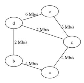
The answer is yes: a can split its stream of data, and send 4Mb/s to c and 2Mb/s to b. The node b relays the 2Mb/s stream of data that it receives from a to d, while node c splits the 4Mb/s stream that it receives into two parts: it relays 3Mb/s of
