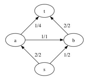
The flow has size 3, which was not optimal (can you see that a flow of size 4 exists?), but if we look at the three possible paths from s to t, that is,  $s \to a \to t$ ,  $s \to a \to t$ , and  $s \to b \to t$ , they each involve an edge used at full capacity.
