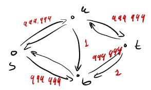
Edmonds-Karp algorithm Ford-Fulkerson, with BFS used to find path in residual network
